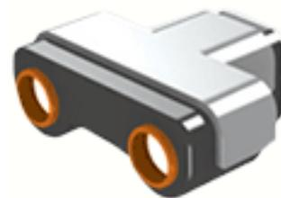
**The Ultrasonic Sensor** is one of the two sensors that give your robot vision [The Light Sensor is the other]. The Ultrasonic Sensor enables your robot to detect objects and to measure the distance to them. You can also use it to make your robot avoid obstacles and detect movement.
